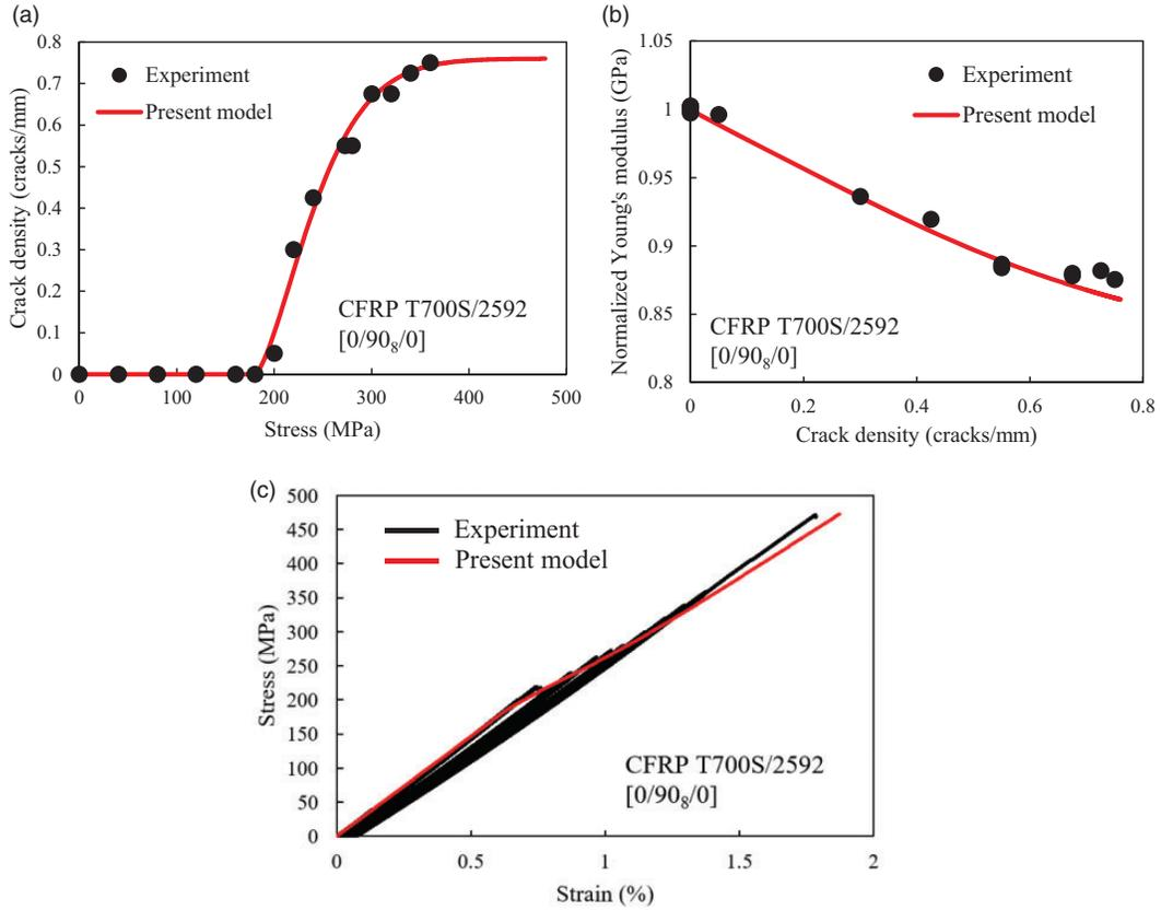
**Figure 11.** Comparison of results predicted using present model for (a) transverse crack density evolution, (b) stiffness reduction, and (c) stress–strain response of T700S/2592 [0/90<sub>8</sub>/0] laminate with experimental results.
