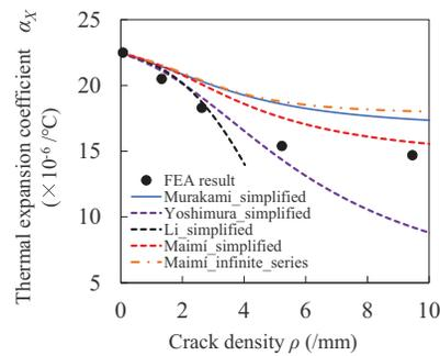
**Figure 9.** Comparison of axial laminate thermal expansion coefficient reduction in GFRP  $[\pm 55]_N$  due to transverse cracking predicted by present models and FEA (Gudmundson and Zhang (1993)).
