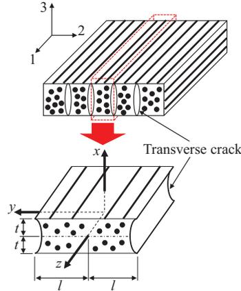
**Figure 1.** Representative volume element in a cracked ply with transverse crack spacing  $2l$  and ply thickness  $2t$ .  $(1, 2, 3)$  is the material coordinate system, and  $(x, y, z)$  is the representative volume element coordinate system.
