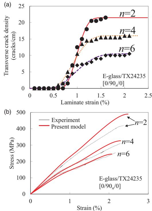
**Figure 13.** Comparison of (a) transverse cracking progression and (b) stress-strain responses of E-glass/TX24235 GFRP  $[0/90_n/0]_s$  ( $n = 2, 4, \text{ and } 6$ ) laminates predicted using the present model with experimental results (Okabe et al. (2004)).
