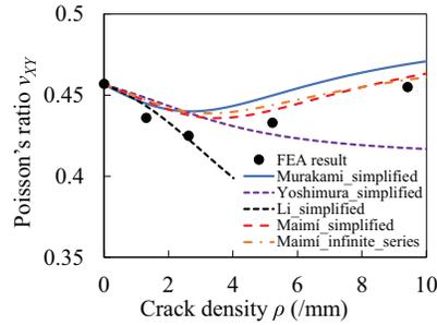
**Figure 8.** Comparison of Poisson's ratio change in GFRP  $[\pm 55]_N$  laminate due to transverse cracking predicted by present models and FEA (Gudmundson and Zhang (1993)).
