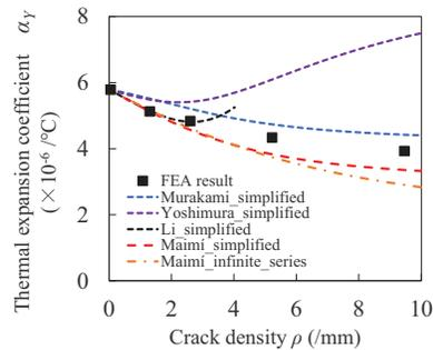
**Figure 10.** Comparison of transverse laminate thermal expansion coefficient reduction in GFRP  $[\pm 55]_N$  due to transverse cracking predicted by present models and FEA (Gudmundson and Zhang (1993)).
