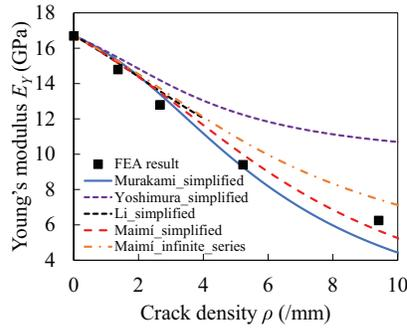
**Figure 6.** Comparison of Young’s moduli reduction in GFRP  $[\pm 55]_N$  transverse laminate due to transverse cracking predicted by present models and FEA (Gudmundson and Zhang (1993)).
