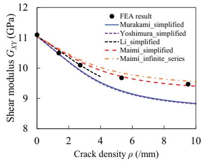
**Figure 7.** Comparison of shear modulus reduction in GFRP  $[\pm 55]_N$  laminate due to transverse cracking predicted by present models and FEA (Gudmundson and Zhang (1993)).
