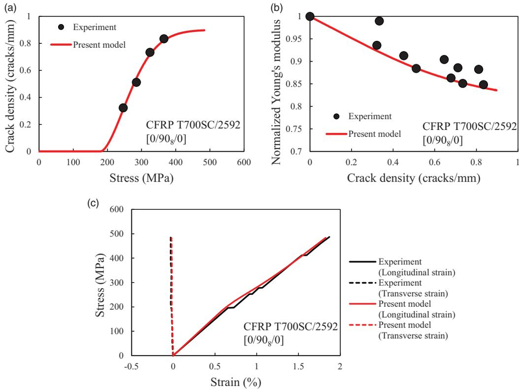
**Figure 12.** Comparison of (a) transverse crack density, (b) stiffness reduction, and (c) stress-strain response of T700SC/2592 [0/90<sub>8</sub>/0] predicted using the present model with experimental results (Fikry et al. (2018)).
