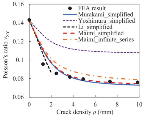
**Figure 4.** Comparison of Poisson's ratio reduction in GFRP  $[90/0]_s$  due to transverse cracking predicted using present models and FEA (Gudmundson and Zhang (1993)).
