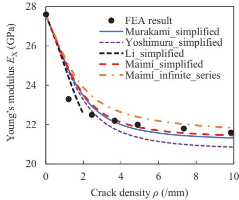
**Figure 3.** Comparison of Young's modulus reduction in GFRP  $[90/0]_s$  laminate due to transverse crack predicted using present models and FEA (Gudmundson and Zhang (1993)).
