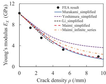
**Figure 5.** Comparison of Young's moduli of GFRP  $[\pm 55]_N$  axial laminates due to transverse cracking predicted by present models and FEA (Gudmundson and Zhang (1993)).
